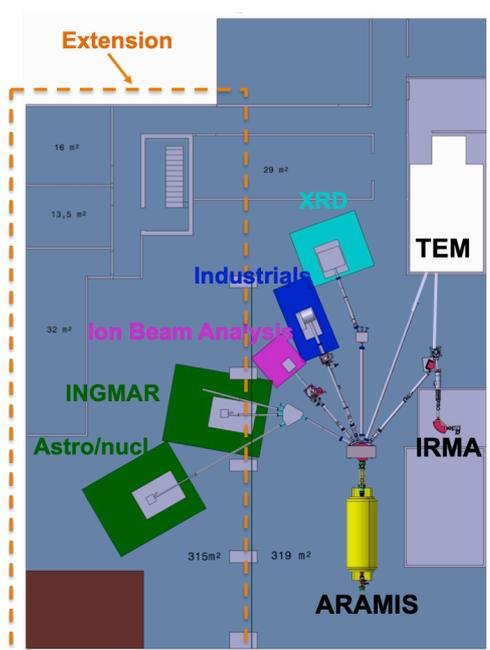
Figure 6 - Scheme of the experimental hall after building extension, showing the different ion beam lines (existing or to be constructed) – the new part is highlighted in orange.
