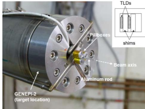
Used to measure gamma heating in low power reactors (mixed gamma-neutron field)
