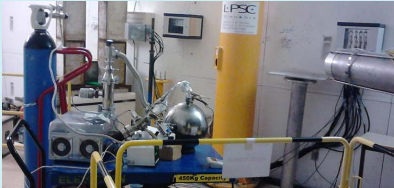
Test of **MIMAC FASTn** (LPSC): directional spectrometer for fast neutrons developed by LPSC : recoil  ${}^4\text{He}$  analysis (elastic scattering)
