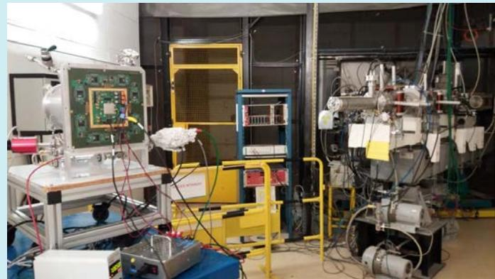
Test of **diamond detectors** for neutron detection (Monodiam, LPSC)
