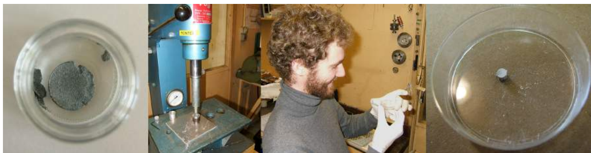
Figure 13: Pellet preparation from reduced \text{TiO}_2 in 2008
